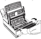
4. Take the new image drum unit out of its package and insert it into your fax machine. To ensure that the image drum is positioned correctly, press down firmly on both of the locations on the image drum marked "PUSH."
